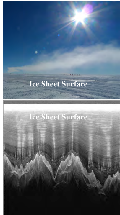
Image (7 top) The East Antarctic ice sheet and a radar image (7 bottom). Radar allows us to see through the ice layers to mountains ~2000 m below!
