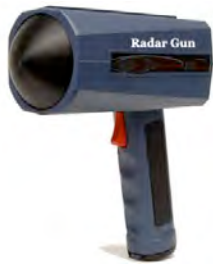
Image 4) The radar gun pictured here is used to measure speed of a baseball pitch.
