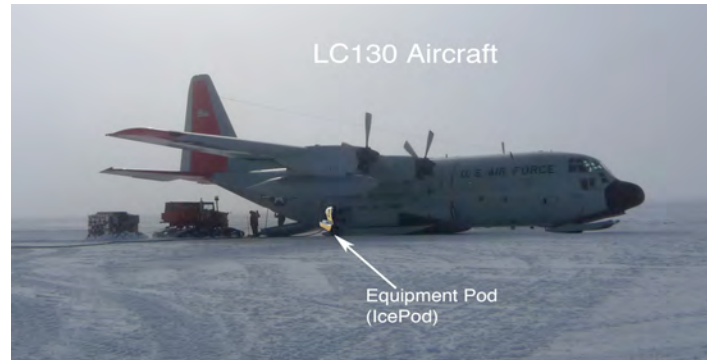
Image 5) The Ice Pod project LC130 Aircraft outfitted with radar mounted on an external 'pod' to collect images of the ice layers and the bedrock surface below. (edited image by R. Bell)
